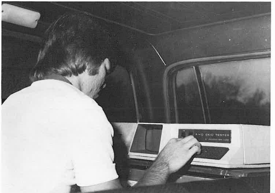
Ron Small enters data into skid unit computer prior to a test run.
