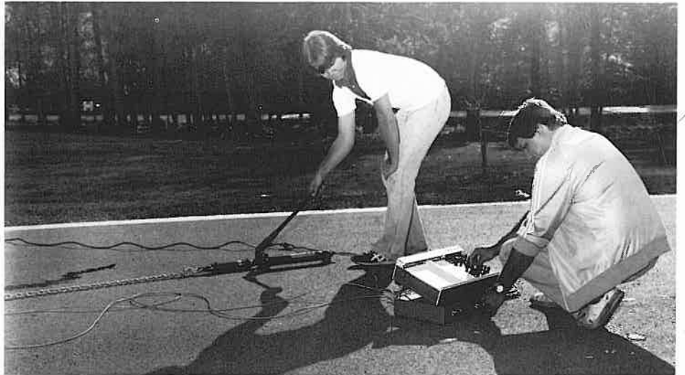
Ron Small operates hydraulic pump to exert pressure on skid unit wheel as Ray Gauer records data.
