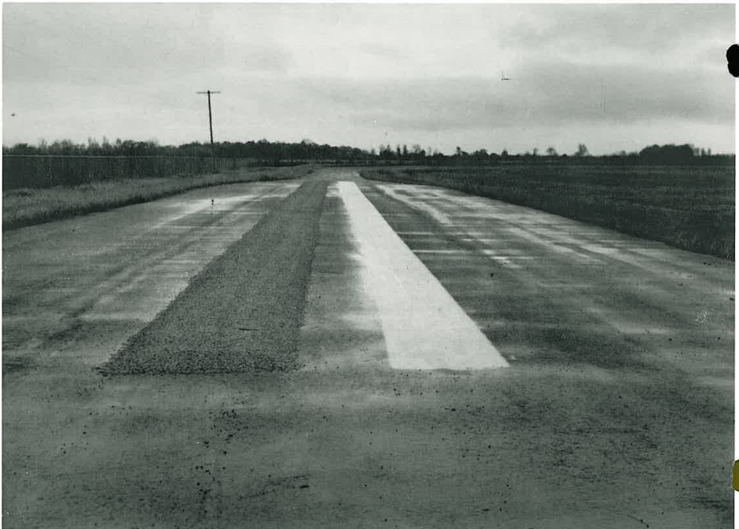
Skid pad provides different surface textures for calibrating the units.
